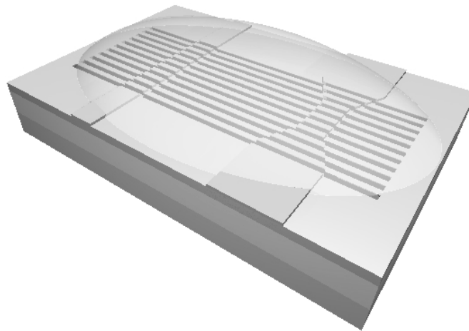
Figure 2.27: Artist impression of a polymer drop applied as a top cladding on the grating regions.
