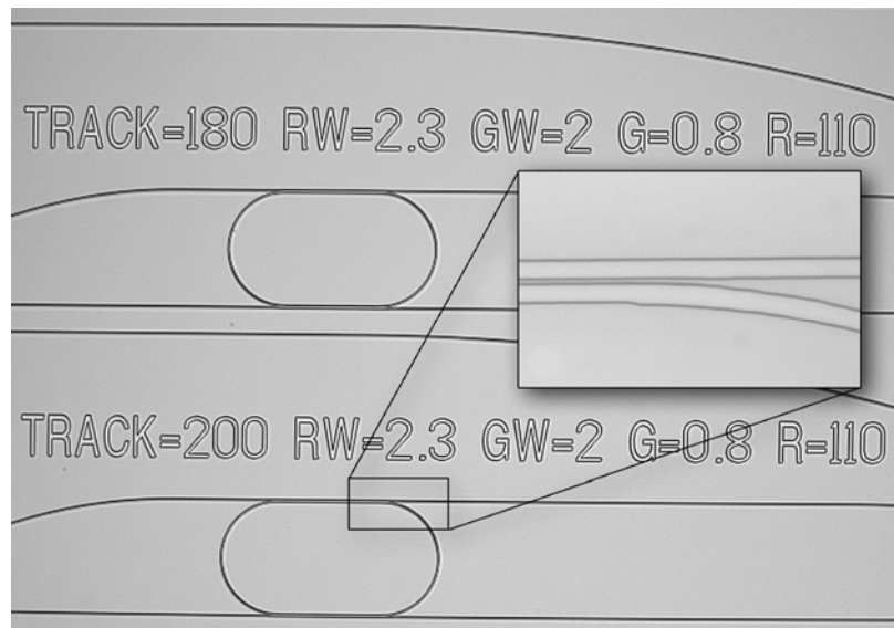
Figure 2.19: Microscope image of laterally coupled \text{Si}_3\text{N}_4 racetrack resonators. The inset shows a detailed view of the transition from bend to straight waveguide of a racetrack with a gap of 800nm.
